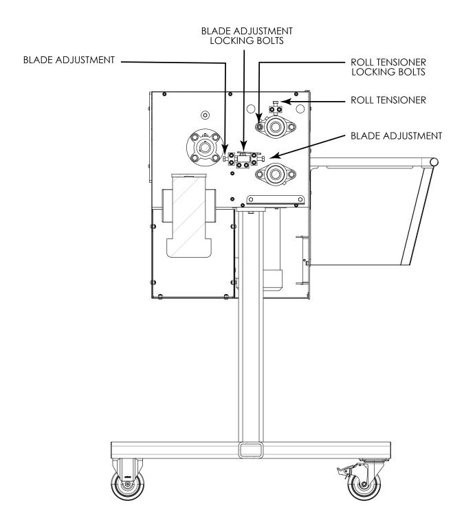
If the rollers do not draw stems into the machine, or following a device rebuild or roller replacement, the rollers must be tensioned to ensure proper preload.
